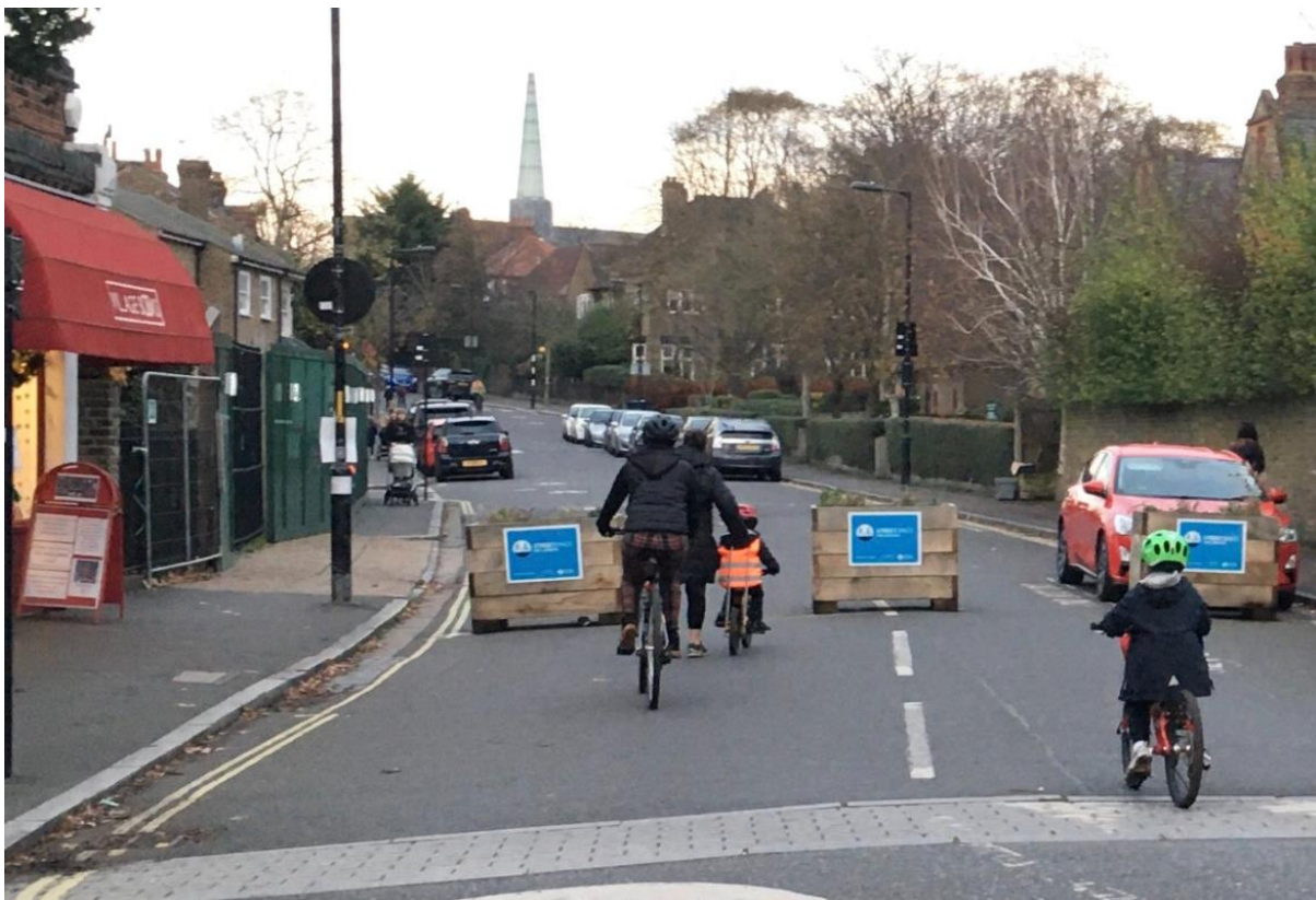
Figure 1: Modal filter planters at the Streetspace site
